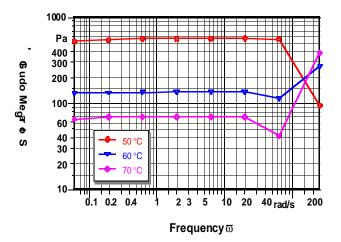
Figure 1. Frequency sweep of cross-linked aqueous gelatin No. 3 solution (20 w/w % at 50°C) treated for 1 h at different temperatures with 20 ppm formaldehyde.
